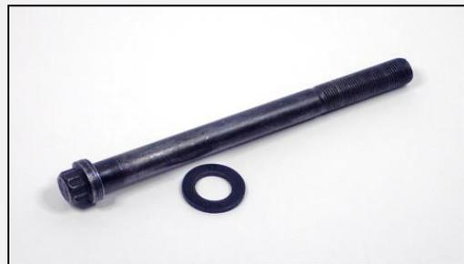
The **MCBN14HBK Head Bolt Kit** consists of thirty-six each of the bolt and washer for complete replacement of all three cylinder heads. Each USA produced bolt features a 170,000 PSI minimum tensile strength specification for greater durability and torque retention and is packed with a thread protector sleeve to prevent damage.
